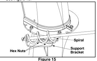
• Adjust the support bracket inward or outward so that the spiral is fully engaged in the notches on the chute before retightening the hex nuts.
